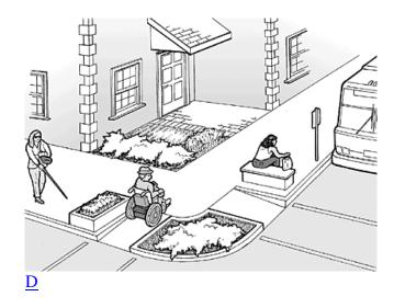
Installation of curb ramps is one of the items included in the transition plan. This type of curb ramp is used when some type of barrier prevents pedestrians from entering the curb ramp from the side.
